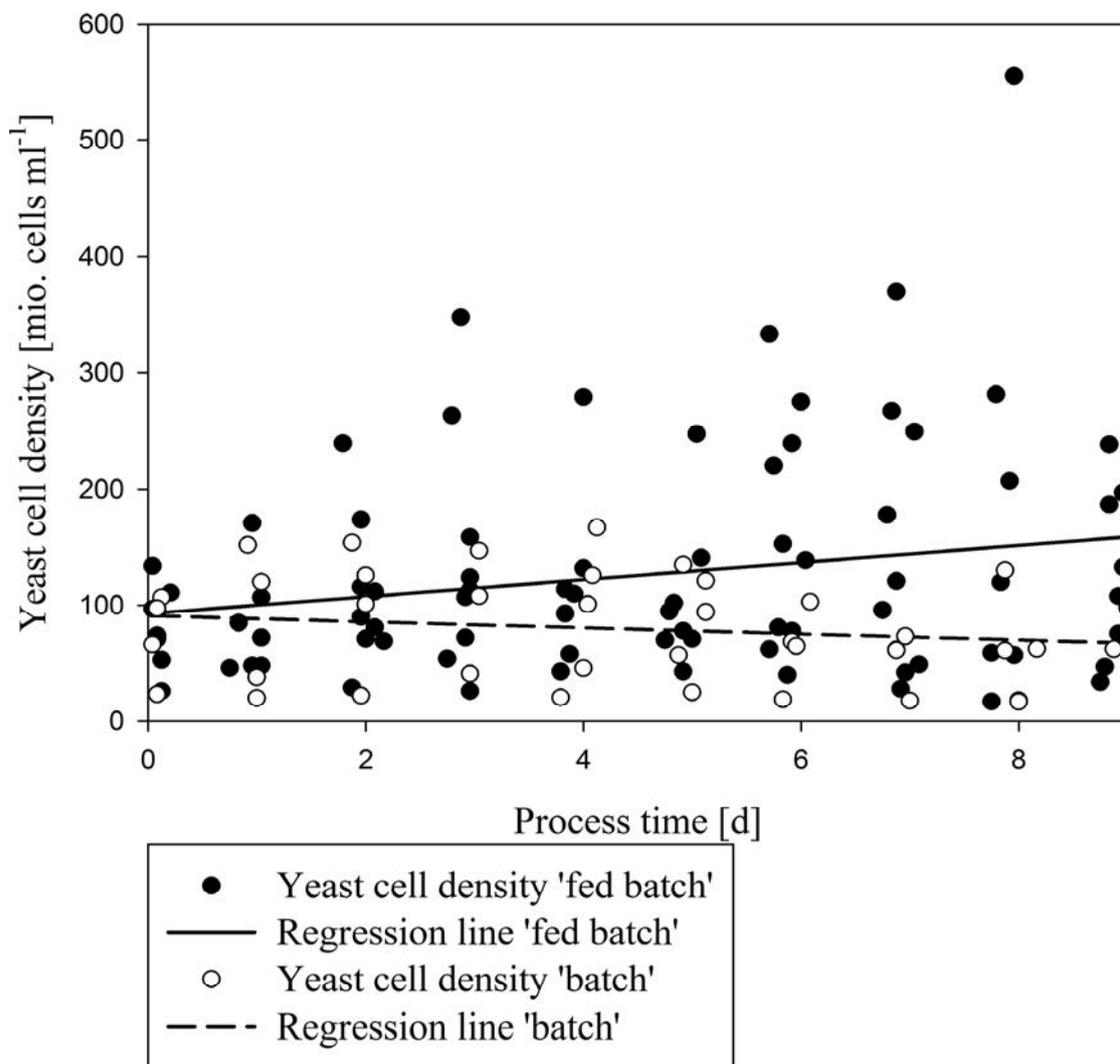
Fig. 2. Yeast cell density recorded in batch and fed-batch bioreactor cultures and regression lines.
