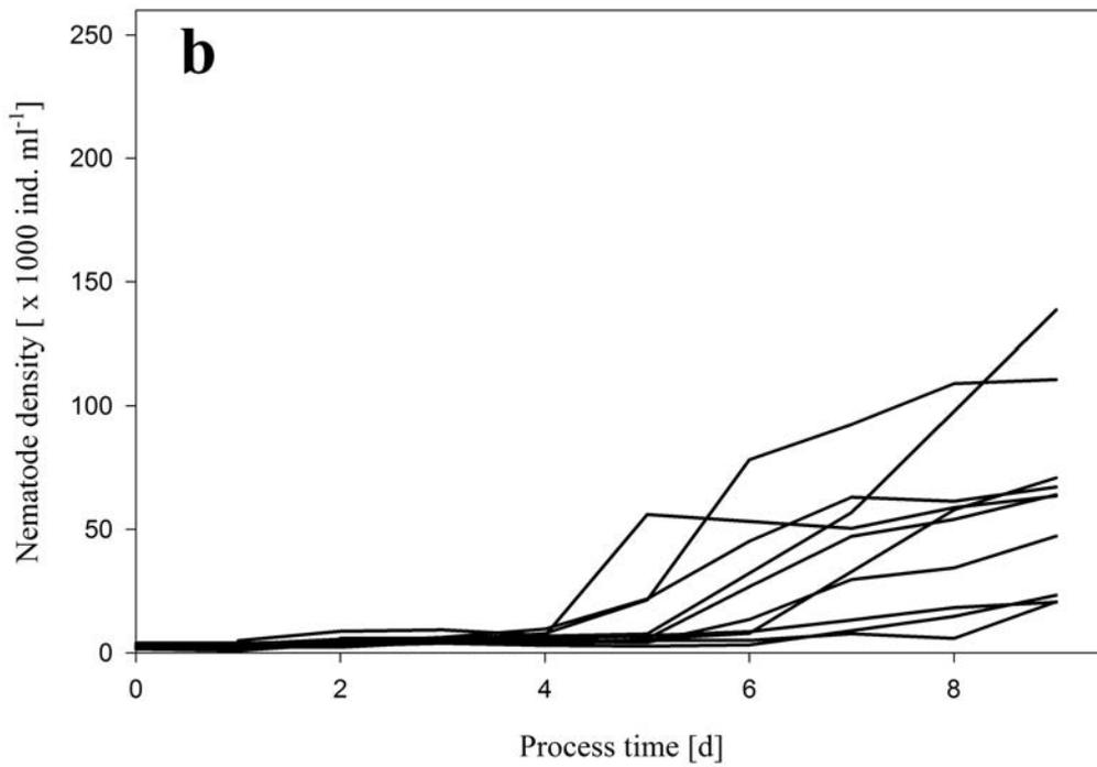
**Fig. 3.** Nematode population density in bioreactors recorded in batch (a; n = 5) and fed-batch (b; n = 10) cultures.
