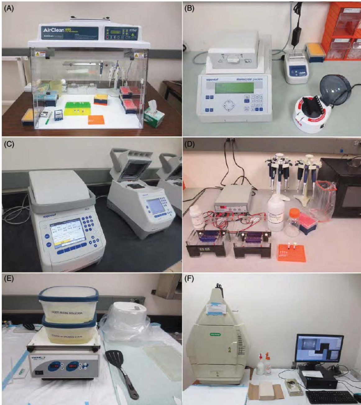
Fig. 12.1. Laboratory equipment. (A) AirClean PCR workstation for preparation of PCR mixture. (B, C) Eppendorf PCR thermocycles. (D) Gel electrophoresis supplies and equipment. (E) Containers for EtBr staining. (F) Bio-Rad gel imaging system.
